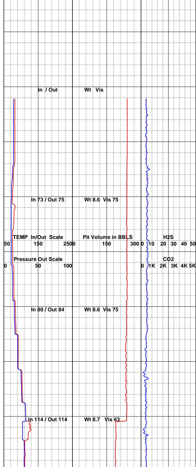
08/22/2014. Hole was previously drilled with 40" bit to 110' and 30" conductor was set to 110' (KB). Drilled out of conductor with 12.25" bit. All depths are referenced from 15' kelly bushing. Hole depth is determined by driller's pipe tally. Sample interval 20'. ROP scale changes @ 2230' & 2630'.
